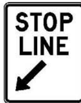
STOP LINE RC-4 L/R 600mm x 750mm
