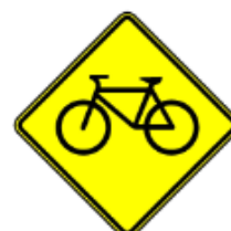
BICYCLE CROSSING AHEAD WC-7 600mm x 600mm
