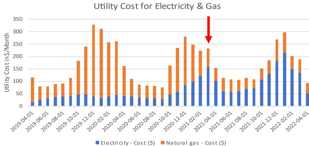
Utility costs for natural gas and electricity for ID #028. The red arrow indicates when the heat pump was installed. A spike occurred in BC Hydro billing at the time of heat pump installation, likely due to fees for BC Hydro equipment upgrades required to support a heat pump. This cost was removed from the data to limit the analysis to operating costs.
