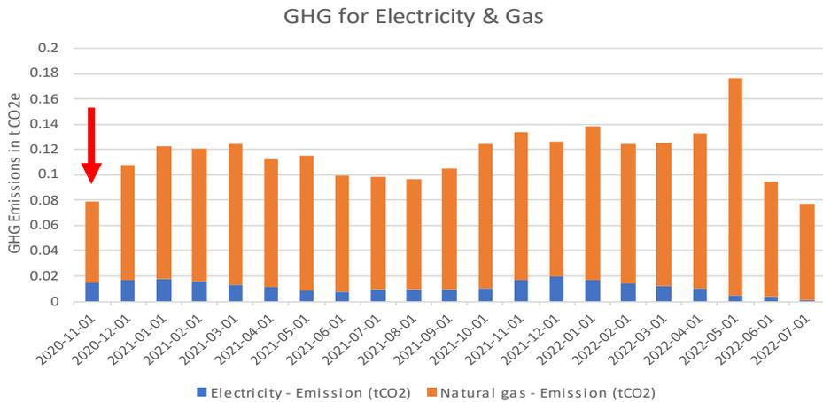
Greenhouse gas (GHG) emissions for natural gas and electricity for ID #008. The red arrow indicates when the heat pump was installed.
