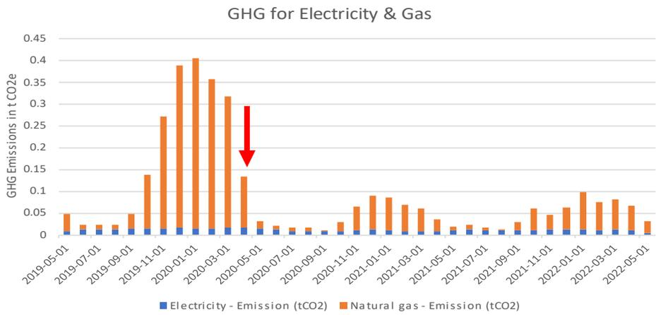
Greenhouse gas (GHG) emissions for natural gas and electricity for ID #004. The red arrow indicates when the heat pump was installed.
