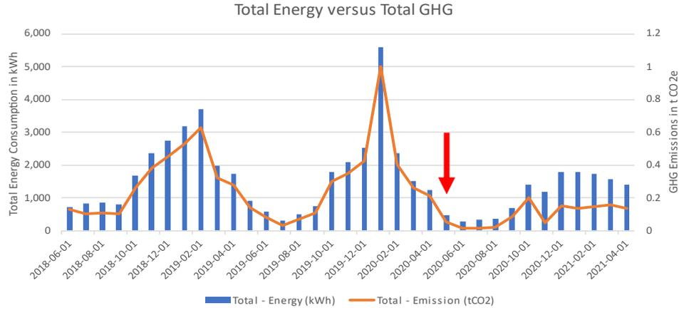
Total energy consumption and greenhouse gas (GHG) emissions for ID #007. The red arrow indicates when the heat pump was installed.
