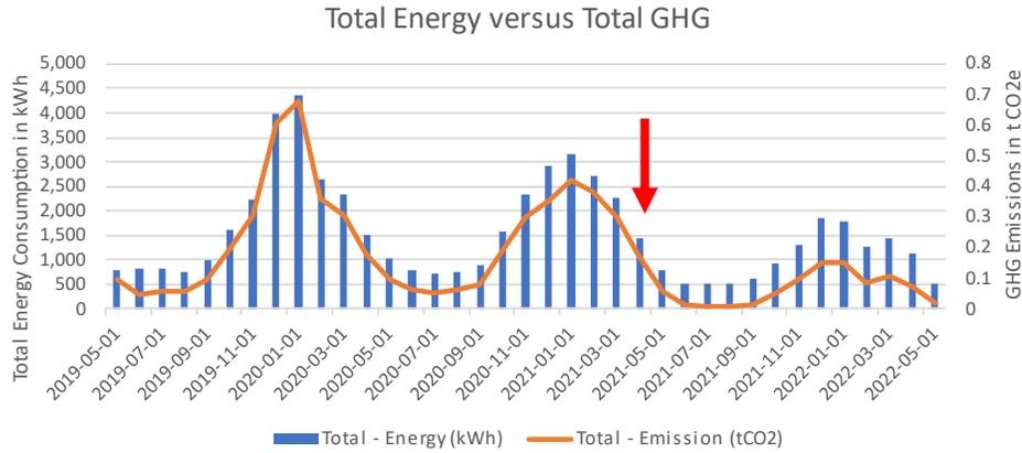
Total energy consumption and greenhouse gas (GHG) emissions for ID #015. The red arrow indicates when the heat pump was installed.
