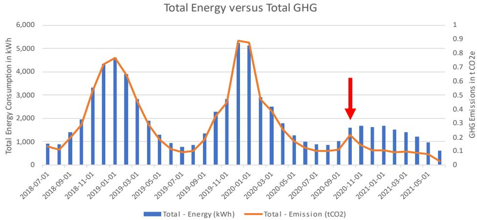
Total energy consumption and greenhouse gas (GHG) emissions for ID #009. The red arrow indicates when the heat pump was installed. There is a notable dip in energy consumption going into winter months when the heat pump is installed.
