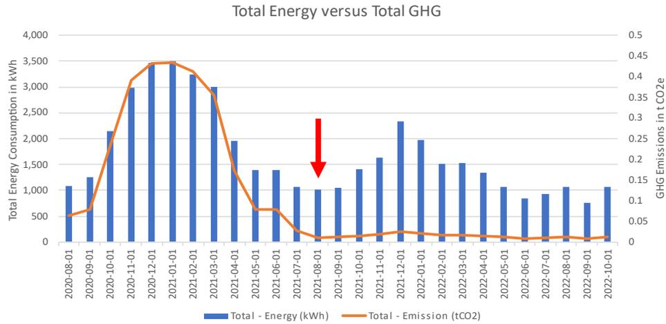
Total energy consumption and greenhouse gas (GHG) emissions for ID #016. The red arrow indicates when the heat pump was installed.
