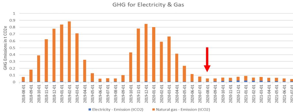
Greenhouse gas (GHG) emissions for natural gas and electricity for ID #001. The red arrow indicates when the heat pump was installed.
