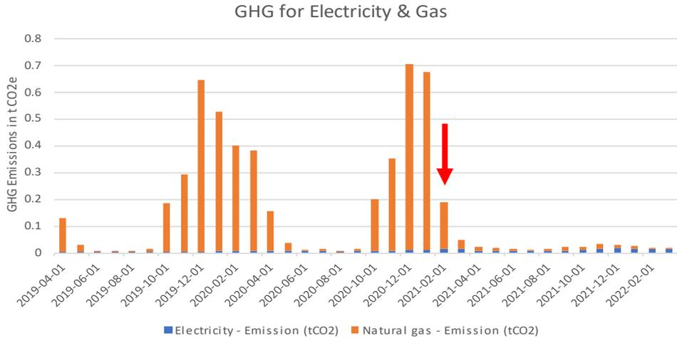
Greenhouse gas (GHG) emissions for natural gas and electricity for ID #002. The red arrow indicates when the heat pump was installed.
