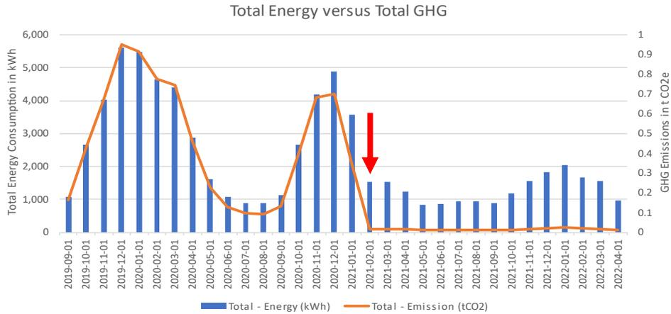
Total energy consumption and greenhouse gas (GHG) emissions for ID #012. The red arrow indicates when the heat pump was installed.
