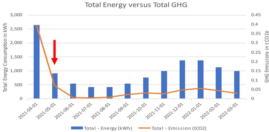
Total energy consumption and greenhouse gas (GHG) emissions for ID #005. The red arrow indicates when the heat pump was installed.
