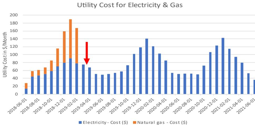
Utility costs for natural gas and electricity for ID #003. The red arrow indicates when the heat pump was installed.
