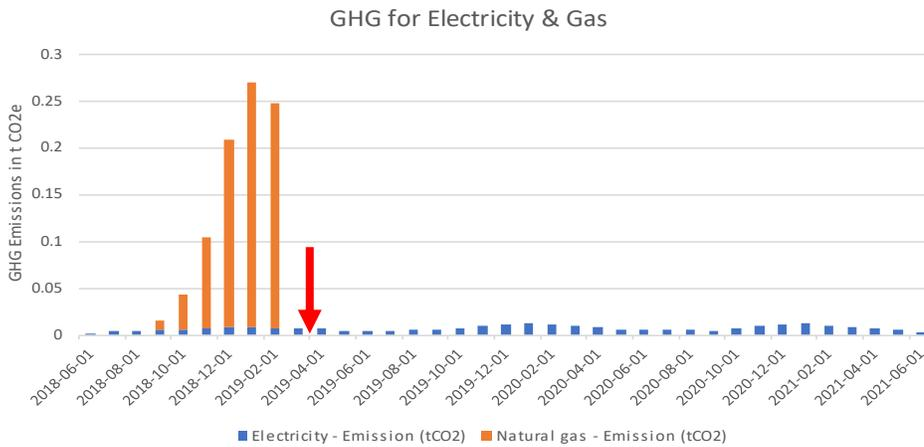
Greenhouse gas (GHG) emissions for natural gas and electricity for ID #003. The red arrow indicates when the heat pump was installed.
