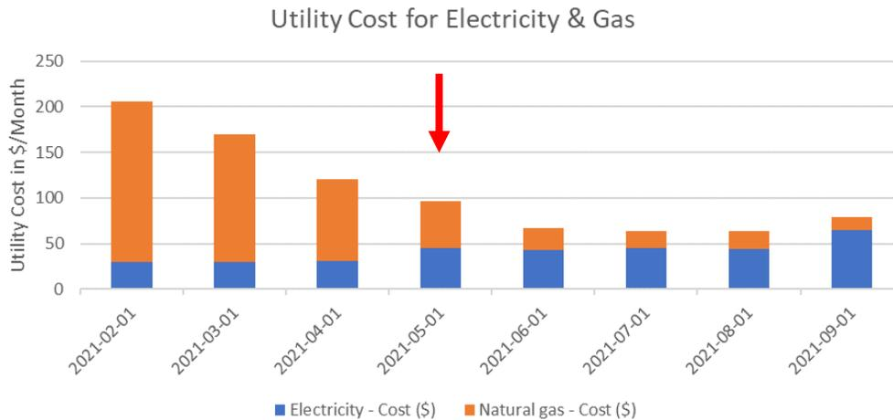
Utility costs for natural gas and electricity for ID #030. The red arrow indicates when the heat pump was installed.
