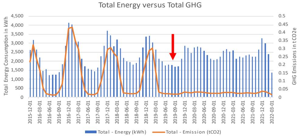
Total energy consumption and greenhouse gas (GHG) emissions for ID #025. The red arrow indicates when the heat pump was installed.
