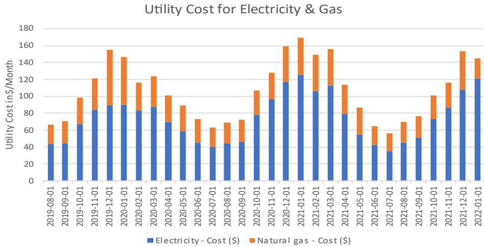
Utility costs for natural gas and electricity for ID #021. The heat pump was installed before the available data begins.
