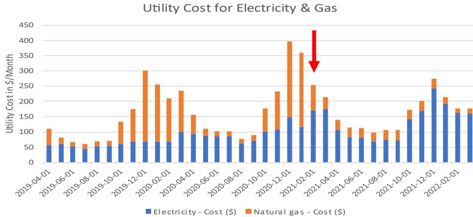
Utility costs for natural gas and electricity for ID #002. The red arrow indicates when the heat pump was installed.
