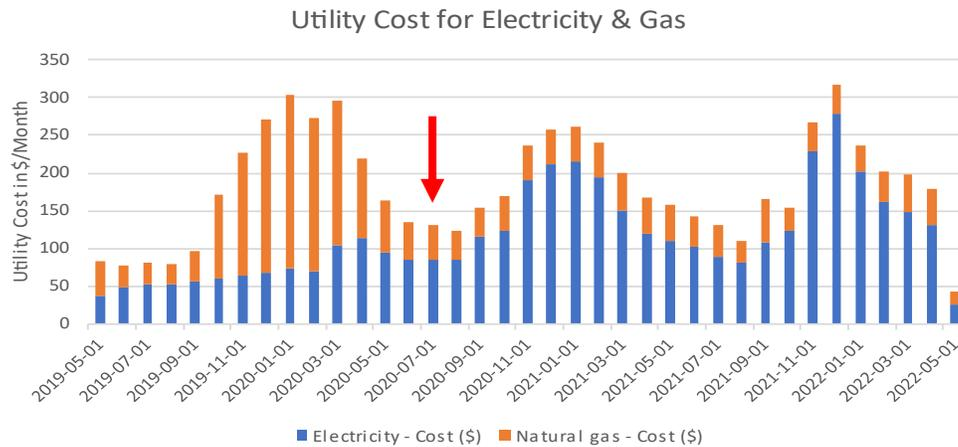
Utility costs for natural gas and electricity for ID #029. The red arrow indicates when the heat pump was installed. A spike occurred in BC Hydro billing at the time of heat pump installation, likely due to fees for BC Hydro equipment upgrades required to support a heat pump. This cost was removed from the data to limit the analysis to operating costs.
