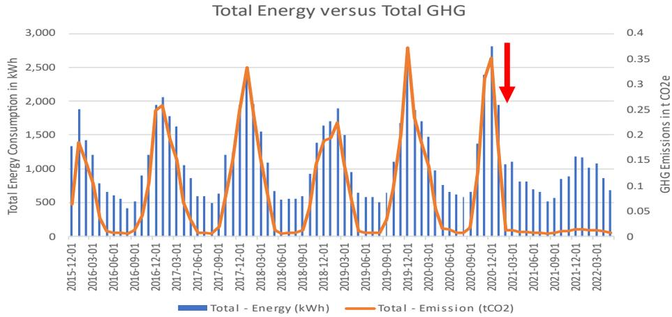
Total energy consumption and greenhouse gas (GHG) emissions for ID #026. The red arrow indicates when the heat pump was installed.
