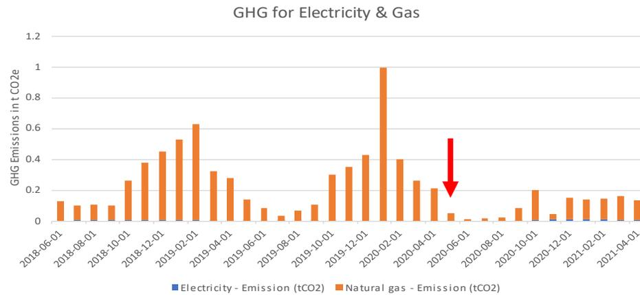
Greenhouse gas (GHG) emissions for natural gas and electricity for ID #007. The red arrow indicates when the heat pump was installed.
