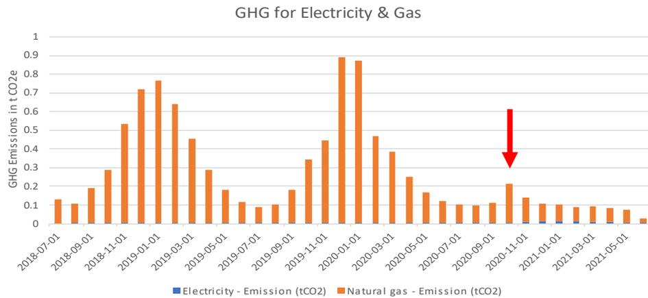
Greenhouse gas (GHG) emissions for natural gas and electricity for ID #009. The red arrow indicates when the heat pump was installed.
