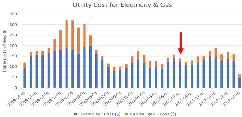
Utility costs for natural gas and electricity for ID #004. The red arrow indicates when the heat pump was installed.
