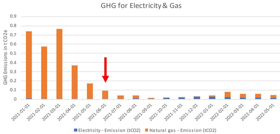
Greenhouse gas (GHG) emissions for natural gas and electricity for ID #006. The red arrow indicates when the heat pump was installed.
