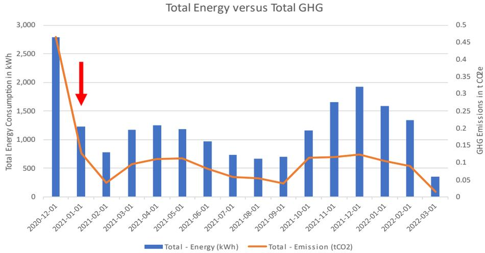
Total energy consumption and greenhouse gas (GHG) emissions for ID #014. The red arrow indicates when the heat pump was installed.
