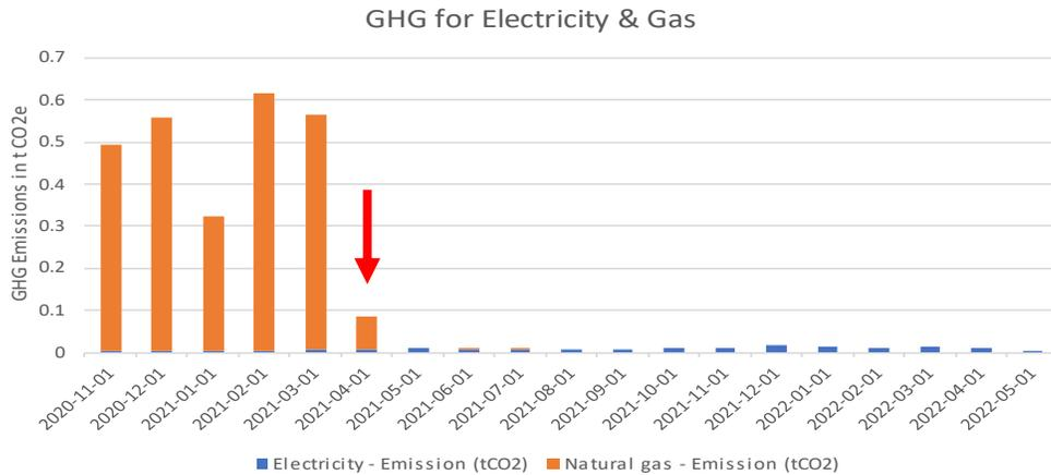
Greenhouse gas (GHG) emissions for natural gas and electricity for ID #013. The red arrow indicates when the heat pump was installed.
