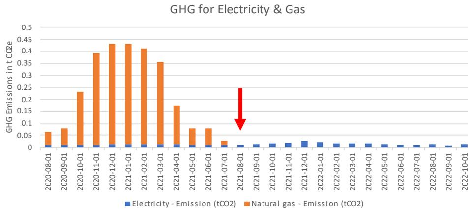
Greenhouse gas (GHG) emissions for natural gas and electricity for ID #016. The red arrow indicates when the heat pump was installed.
