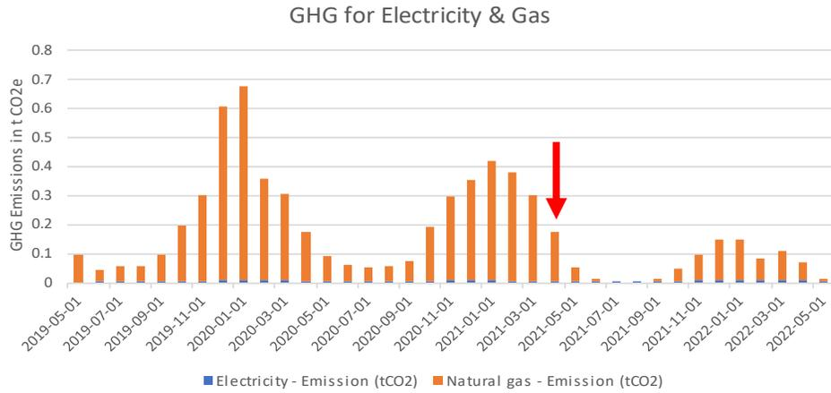
Greenhouse gas (GHG) emissions for natural gas and electricity for ID #015. The red arrow indicates when the heat pump was installed.
