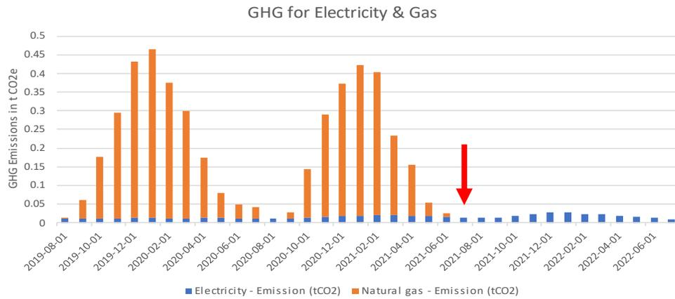
Greenhouse gas (GHG) emissions for natural gas and electricity for ID #020. The red arrow indicates when the heat pump was installed.
