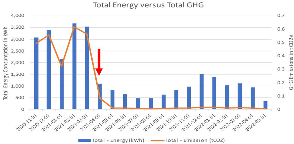
Total energy consumption and greenhouse gas (GHG) emissions for ID #013. The red arrow indicates when the heat pump was installed.
