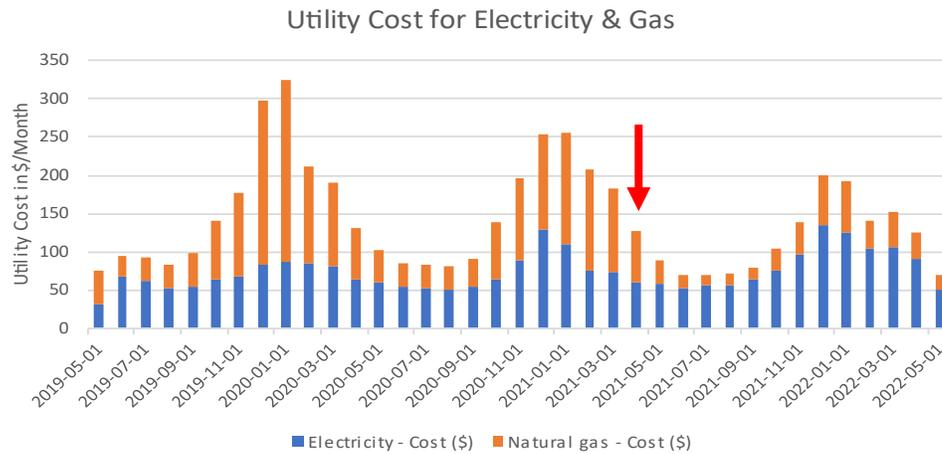
Utility costs for natural gas and electricity for ID #015. The red arrow indicates when the heat pump was installed.
