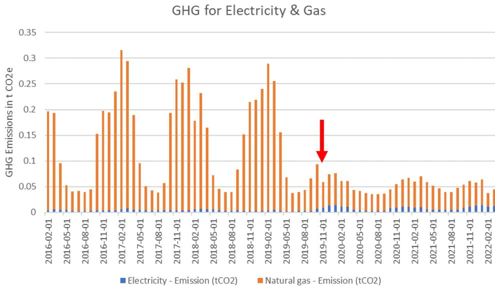
Figure 2: Greenhouse gas (GHG) emissions for natural gas (orange) and electricity (blue) for ID #018. The red arrow indicates when the heat pump was installed.
