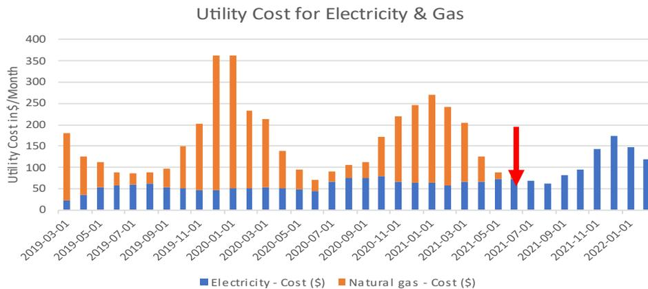
Utility costs for natural gas and electricity for ID #017. The red arrow indicates when the heat pump was installed. A spike occurred in BC Hydro billing at the time of heat pump installation, likely due to fees for BC Hydro equipment upgrades required to support a heat pump. This cost was removed from the data to limit the analysis to operating costs.
