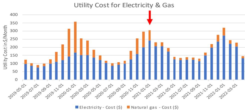
Utility costs for natural gas and electricity for ID #032. The red arrow indicates when the heat pump was installed.
