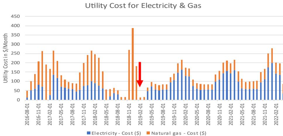
Utility costs for natural gas and electricity for ID #010. The red arrow indicates when the heat pump was installed.
