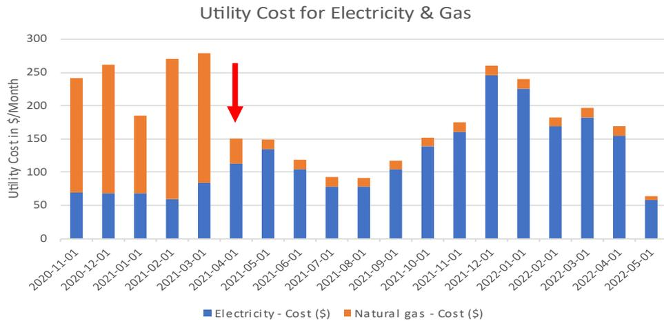
Utility costs for natural gas and electricity for ID #013. The red arrow indicates when the heat pump was installed.
