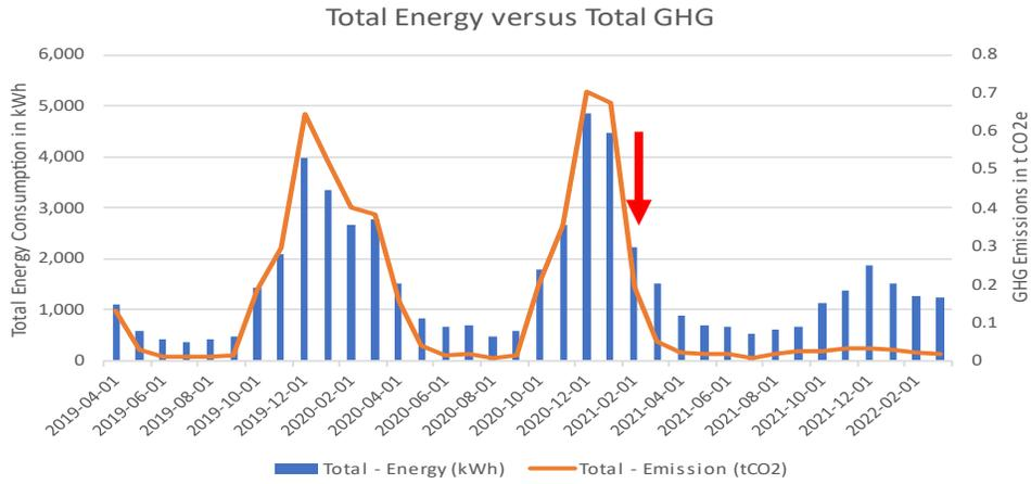
Total energy consumption and greenhouse gas (GHG) emissions for ID #002. The red arrow indicates when the heat pump was installed.
