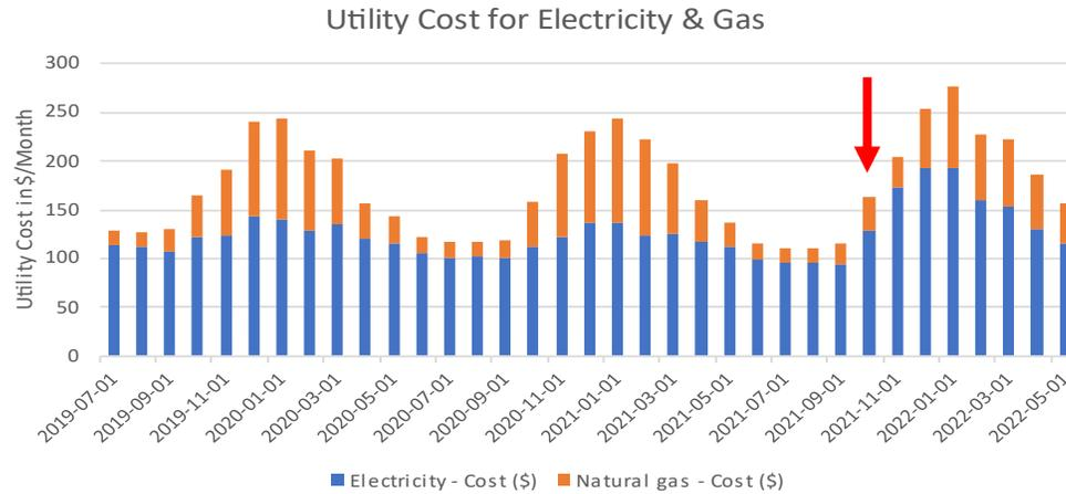
Utility costs for natural gas and electricity for ID #024. The red arrow indicates when the heat pump was installed.
