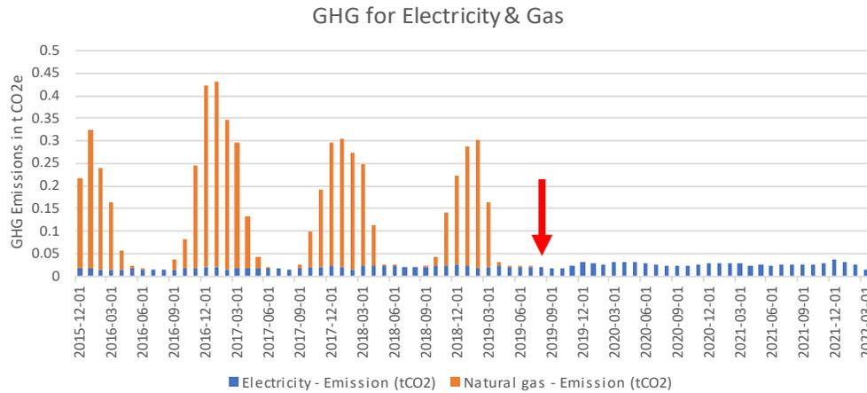
Greenhouse gas (GHG) emissions for natural gas and electricity for ID #025. The red arrow indicates when the heat pump was installed.
