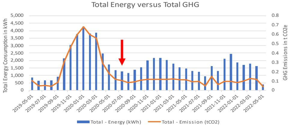
Total energy consumption and greenhouse gas (GHG) emissions for ID #029. The red arrow indicates when the heat pump was installed.
