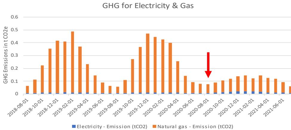
Greenhouse gas (GHG) emissions for natural gas and electricity for ID #023. The red arrow indicates when the heat pump was installed.
