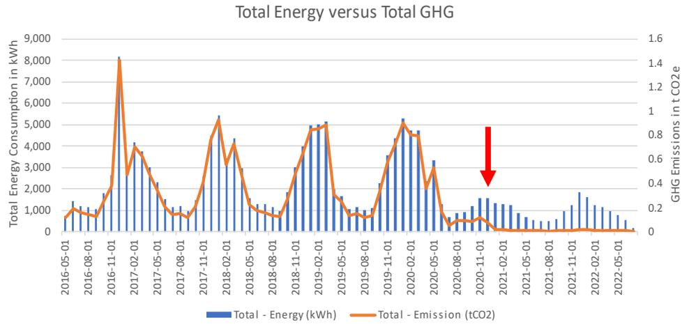
Total energy consumption and greenhouse gas (GHG) emissions for ID #019. The red arrow indicates when the heat pump was installed.
