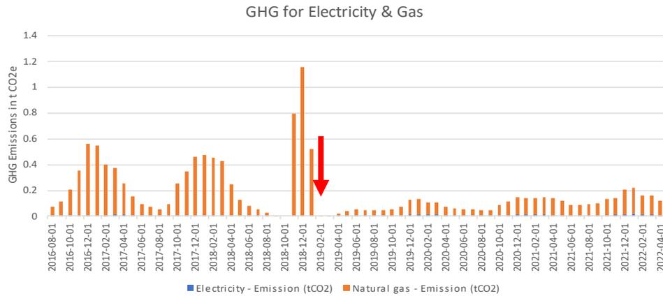
Greenhouse gas (GHG) emissions for natural gas and electricity for ID #010. The red arrow indicates when the heat pump was installed.
