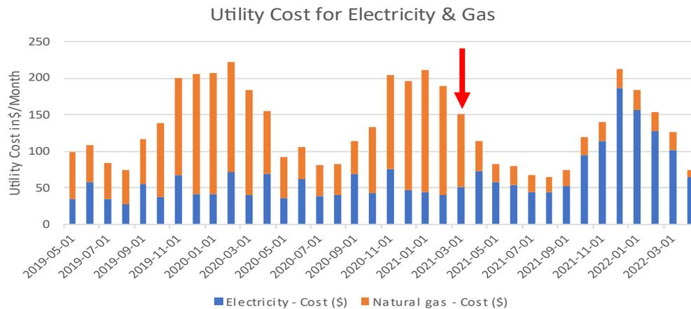
Utility costs for natural gas and electricity for ID #031. The red arrow indicates when the heat pump was installed. Note that BC Hydro bill costs were not provided, so electricity costing was calculated by RDH based off of consumption using current BC Hydro rates.
