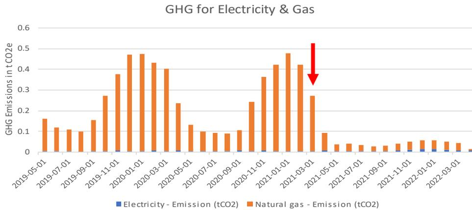
Greenhouse gas (GHG) emissions for natural gas and electricity for ID #031. The red arrow indicates when the heat pump was installed.
