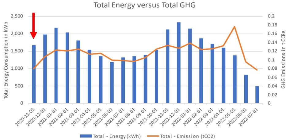
Total energy consumption and greenhouse gas (GHG) emissions for ID #008. The red arrow indicates when the heat pump was installed.
