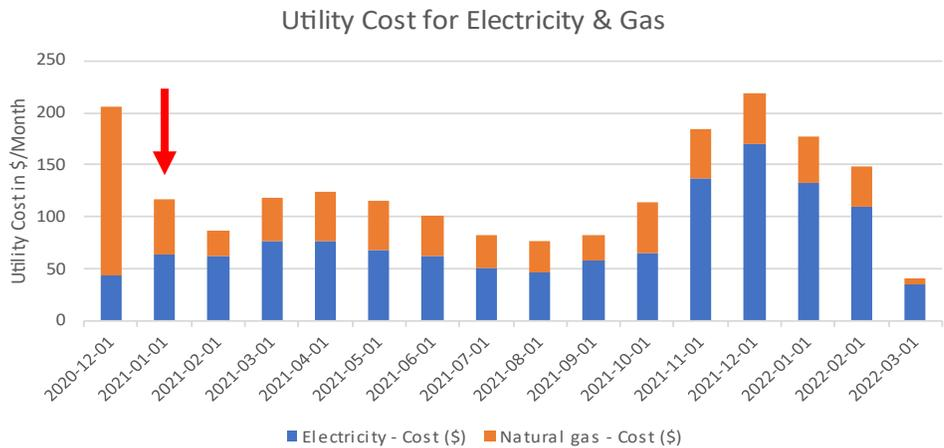
Utility costs for natural gas and electricity for ID #014. The red arrow indicates when the heat pump was installed.
