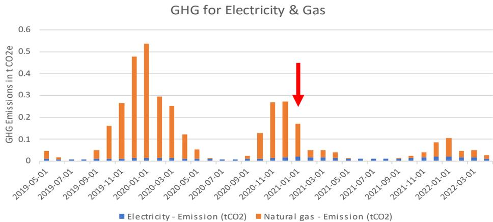
Greenhouse gas (GHG) emissions for natural gas and electricity for ID #032. The red arrow indicates when the heat pump was installed.
