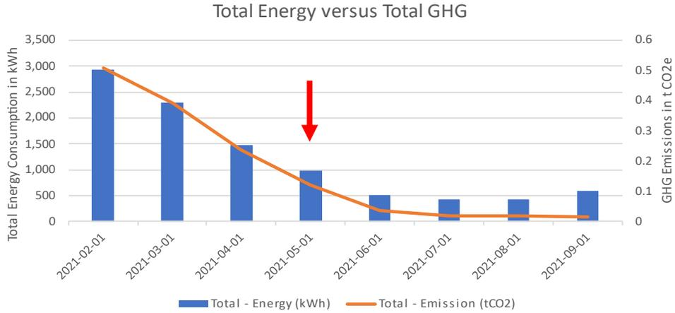
Total energy consumption and greenhouse gas (GHG) emissions for ID #030. The red arrow indicates when the heat pump was installed.
