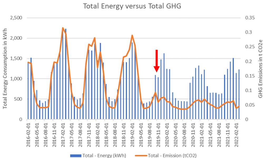
Figure 1: Total energy consumption (blue) and greenhouse gas (GHG) emissions (orange) for ID #018. The red arrow indicates when the heat pump was installed.
