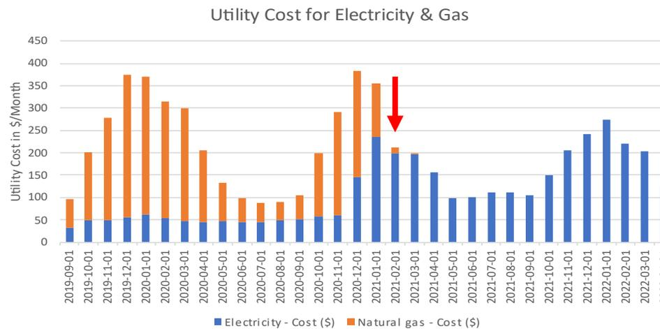
Utility costs for natural gas and electricity for ID #012. The red arrow indicates when the heat pump was installed.
