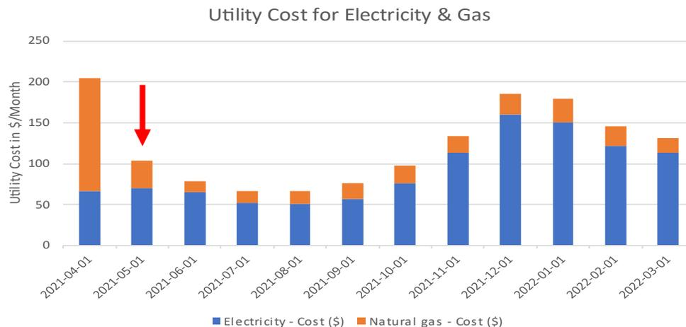
Utility costs for natural gas and electricity for ID #005. The red arrow indicates when the heat pump was installed. Note that BC Hydro bill costs were not provided, so electricity costing was calculated by RDH based off of consumption using current BC Hydro rates.
