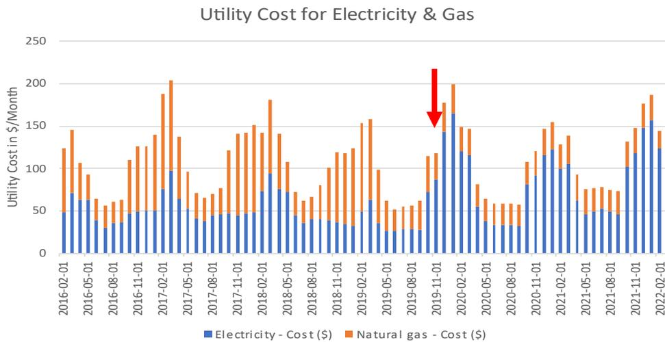
Utility costs for natural gas and electricity for ID #018. The red arrow indicates when the heat pump was installed.
