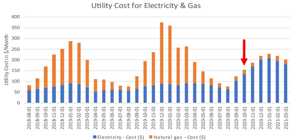
Utility costs for natural gas and electricity for ID #011. The red arrow indicates when the heat pump was installed. A spike occurred in BC Hydro billing at the time of heat pump installation, likely due to fees for BC Hydro equipment upgrades required to support a heat pump. This cost was removed from the data to limit the analysis to operating costs.
