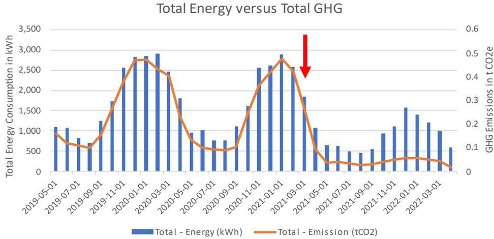
Total energy consumption and greenhouse gas (GHG) emissions for ID #031. The red arrow indicates when the heat pump was installed.
