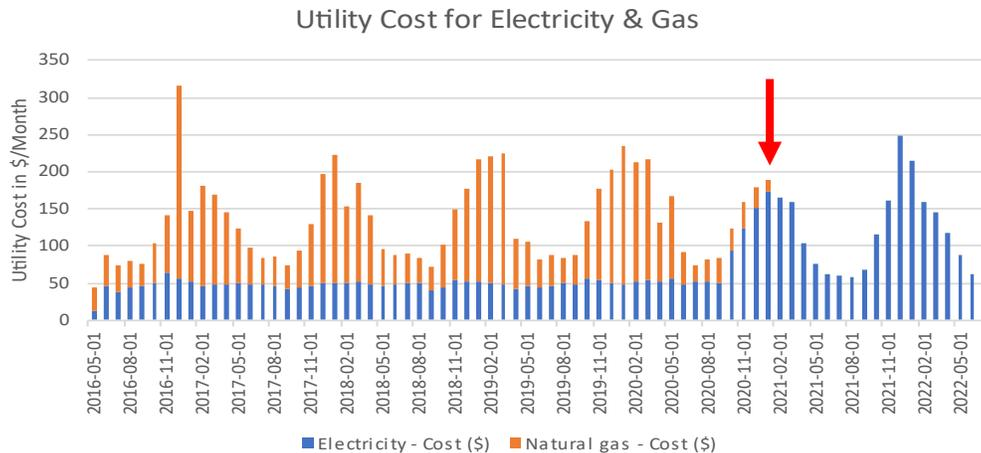
Utility costs for natural gas and electricity for ID #019. The red arrow indicates when the heat pump was installed.
