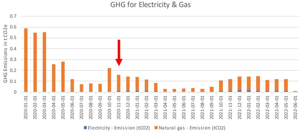
Greenhouse gas (GHG) emissions for natural gas and electricity for ID #022. The red arrow indicates when the heat pump was installed.
