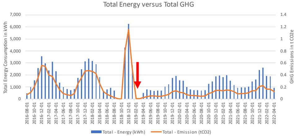
Total energy consumption and greenhouse gas (GHG) emissions for ID #010. The red arrow indicates when the heat pump was installed. There is a gap in the provided data for the 2018/19 winter which makes the data appear to spike abruptly.
