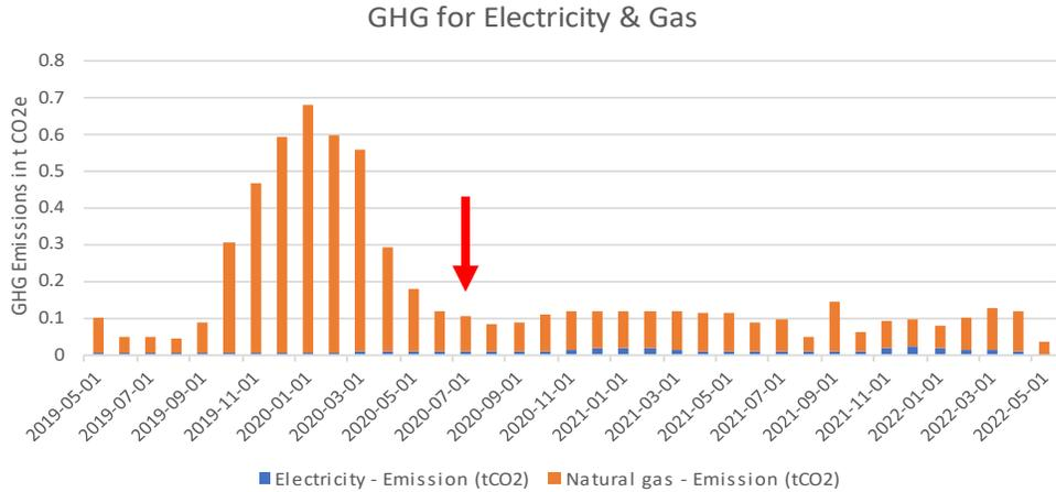
Greenhouse gas (GHG) emissions for natural gas and electricity for ID #029. The red arrow indicates when the heat pump was installed.
