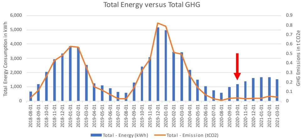
Total energy consumption and greenhouse gas (GHG) emissions for ID #011. The red arrow indicates when the heat pump was installed.
