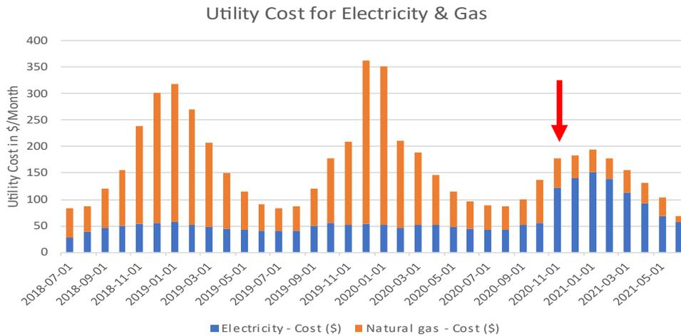
Utility costs for natural gas and electricity for ID #009. The red arrow indicates when the heat pump was installed.
