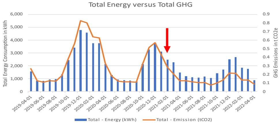
Total energy consumption and greenhouse gas (GHG) emissions for ID #028. The red arrow indicates when the heat pump was installed.
