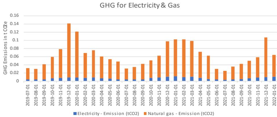
Greenhouse gas (GHG) emissions for natural gas and electricity for ID #021. The heat pump was installed before the available data begins.
