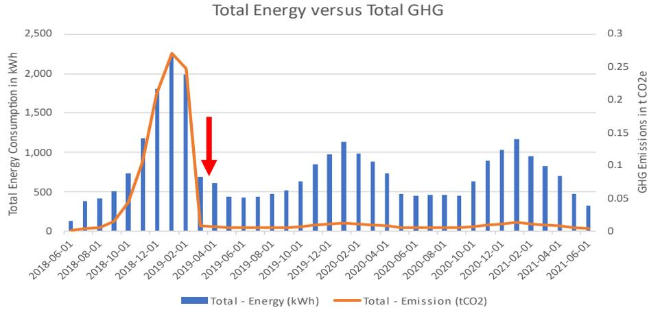
Total energy consumption and greenhouse gas (GHG) emissions for ID #003. The red arrow indicates when the heat pump was installed.
