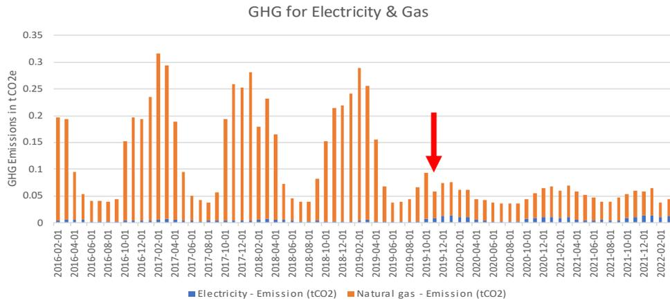
Greenhouse gas (GHG) emissions for natural gas and electricity for ID #018. The red arrow indicates when the heat pump was installed.
