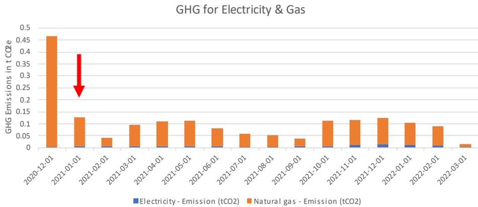
Greenhouse gas (GHG) emissions for natural gas and electricity for ID #014. The red arrow indicates when the heat pump was installed.
