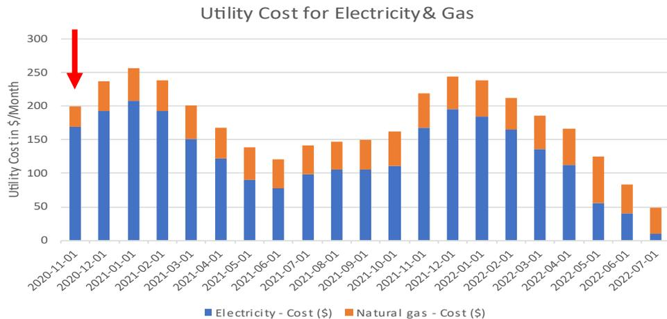
Utility costs for natural gas and electricity for ID #008. The red arrow indicates when the heat pump was installed.
