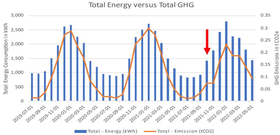
Total energy consumption and greenhouse gas (GHG) emissions for ID #024. The red arrow indicates when the heat pump was installed.
