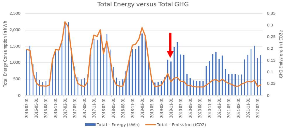
Total energy consumption and greenhouse gas (GHG) emissions for ID #018. The red arrow indicates when the heat pump was installed.
