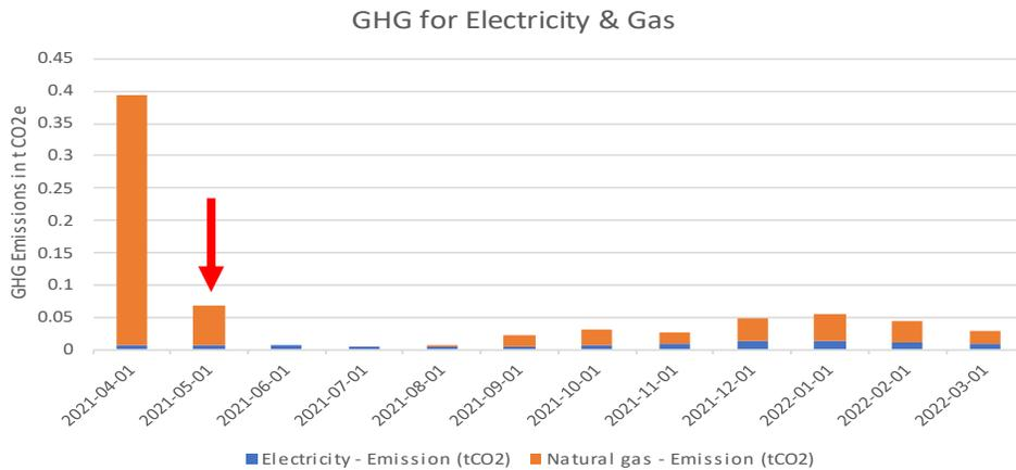
Greenhouse gas (GHG) emissions for natural gas and electricity for ID #005. The red arrow indicates when the heat pump was installed.
