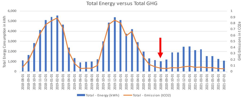
Total energy consumption and greenhouse gas (GHG) emissions for ID #001. The red arrow indicates when the heat pump was installed.
