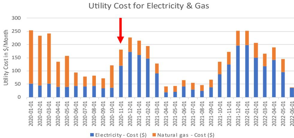
Utility costs for natural gas and electricity for ID #022. The red arrow indicates when the heat pump was installed. Note that BC Hydro bill costs were not provided, so electricity costing was calculated by RDH based off of consumption using current BC Hydro rates.
