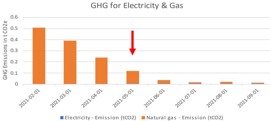
Greenhouse gas (GHG) emissions for natural gas and electricity for ID #030. The red arrow indicates when the heat pump was installed.
