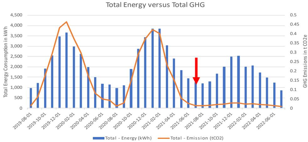
Total energy consumption and greenhouse gas (GHG) emissions for ID #020. The red arrow indicates when the heat pump was installed.
