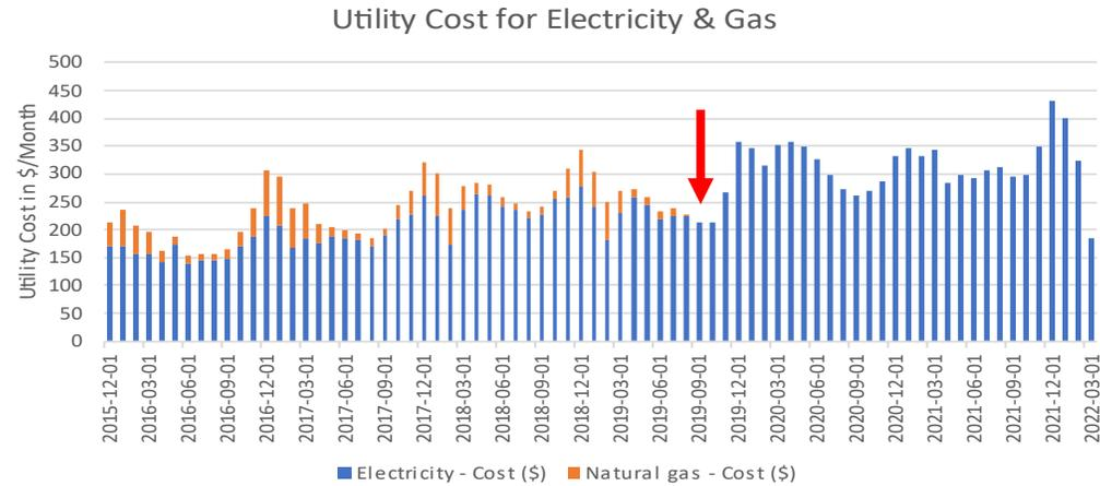
Utility costs for natural gas and electricity for ID #025. The red arrow indicates when the heat pump was installed.
