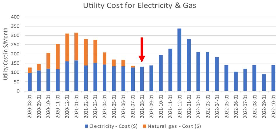
Utility costs for natural gas and electricity for ID #016. The red arrow indicates when the heat pump was installed. Note that BC Hydro bill costs were not provided, so electricity costing was calculated by RDH based off of consumption using current BC Hydro rates.
