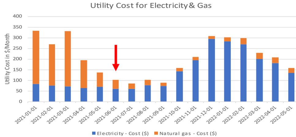
Utility costs for natural gas and electricity for ID #006. The red arrow indicates when the heat pump was installed.
