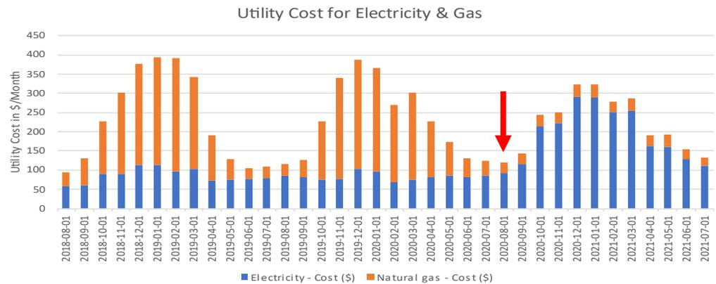
Utility costs for natural gas and electricity for ID #001. The red arrow indicates when the heat pump was installed.
