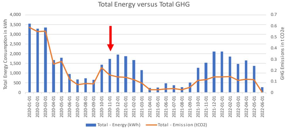
Total energy consumption and greenhouse gas (GHG) emissions for ID #022. The red arrow indicates when the heat pump was installed.
