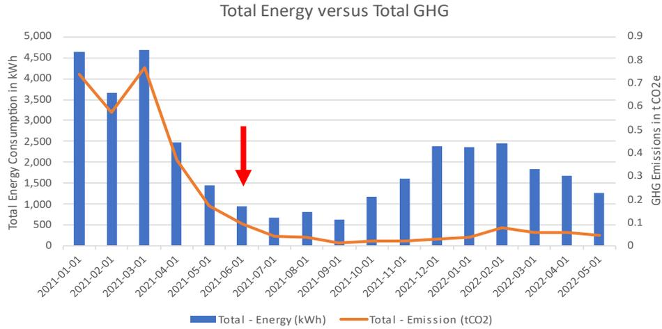
Total energy consumption and greenhouse gas (GHG) emissions for ID #006. The red arrow indicates when the heat pump was installed.
