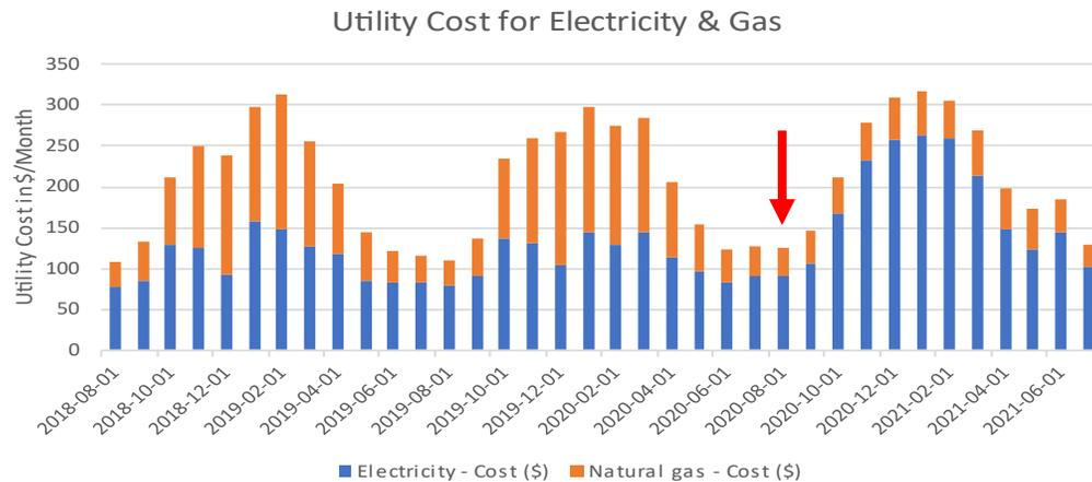
Utility costs for natural gas and electricity for ID #023. The red arrow indicates when the heat pump was installed. Note that BC Hydro bill costs were not provided, so electricity costing was calculated by RDH based off of consumption using current BC Hydro rates.
