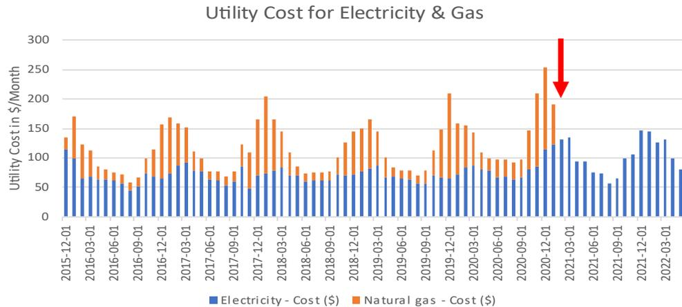
Utility costs for natural gas and electricity for ID #026. The red arrow indicates when the heat pump was installed.
