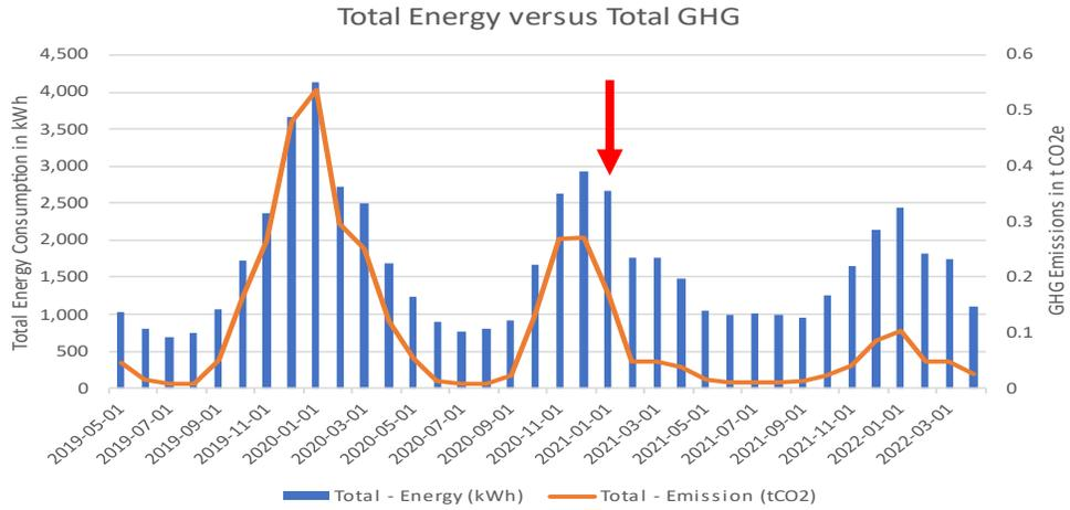
Total energy consumption and greenhouse gas (GHG) emissions for ID #032. The red arrow indicates when the heat pump was installed.
