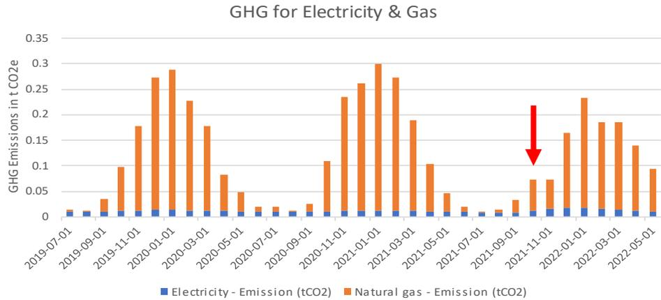
Greenhouse gas (GHG) emissions for natural gas and electricity for ID #024. The red arrow indicates when the heat pump was installed.
