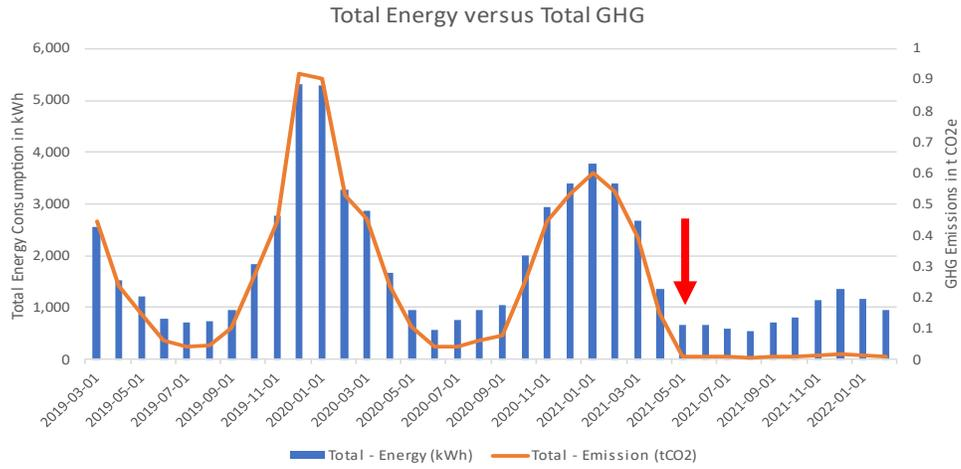
Total energy consumption and greenhouse gas (GHG) emissions for ID #017. The red arrow indicates when the heat pump was installed.
