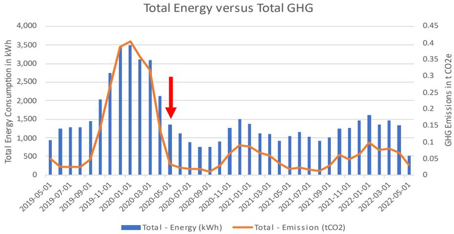
Total energy consumption and greenhouse gas (GHG) emissions for ID #004. The red arrow indicates when the heat pump was installed.
