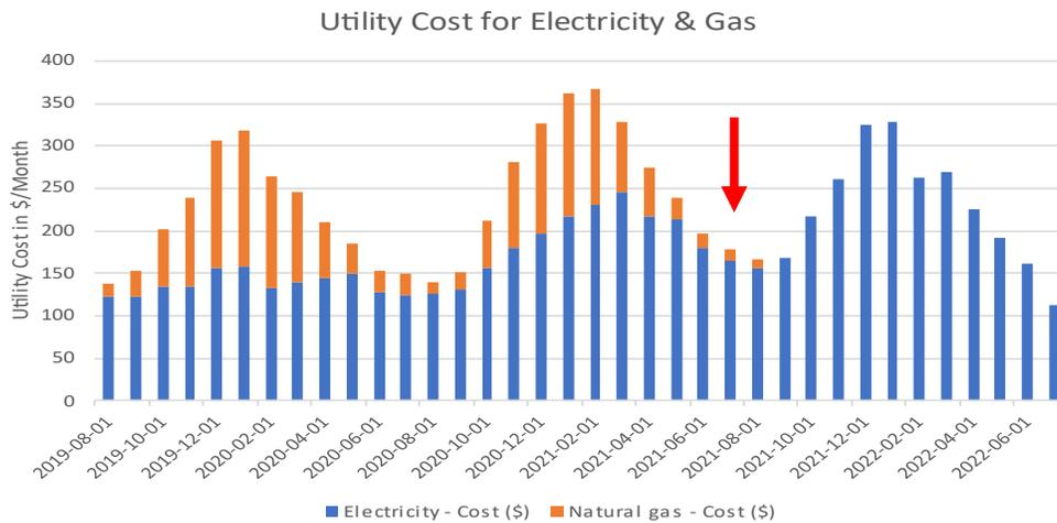
Utility costs for natural gas and electricity for ID #020. The red arrow indicates when the heat pump was installed. Some base charges continue after heat pump installation despite zero natural gas consumption before Fortis BC billing was stopped.
