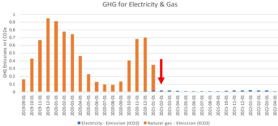
Greenhouse gas (GHG) emissions for natural gas and electricity for ID #012. The red arrow indicates when the heat pump was installed.
