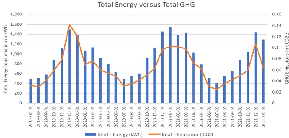
Total energy consumption and greenhouse gas (GHG) emissions for ID #021. The heat pump was installed before the available data begins.
