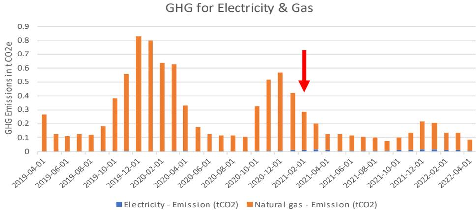
Greenhouse gas (GHG) emissions for natural gas and electricity for ID #028. The red arrow indicates when the heat pump was installed.
