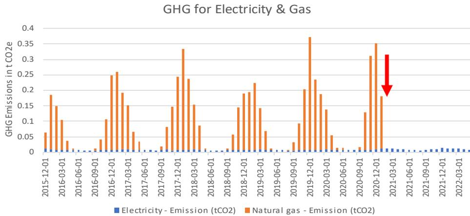
Greenhouse gas (GHG) emissions for natural gas and electricity for ID #026. The red arrow indicates when the heat pump was installed.
