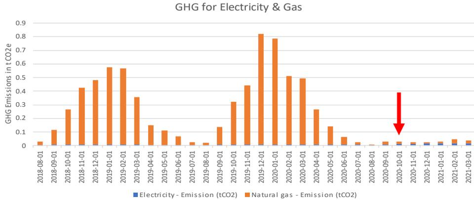
Greenhouse gas (GHG) emissions for natural gas and electricity for ID #011. The red arrow indicates when the heat pump was installed.
