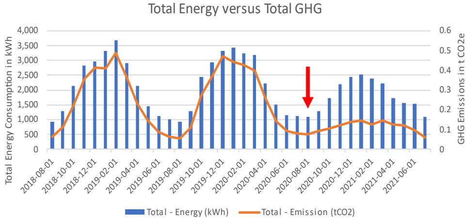
Total energy consumption and greenhouse gas (GHG) emissions for ID #023. The red arrow indicates when the heat pump was installed.
