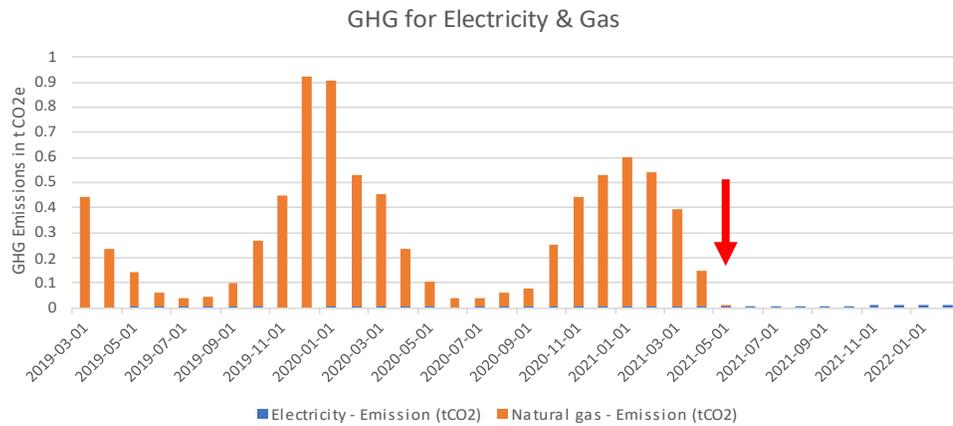
Greenhouse gas (GHG) emissions for natural gas and electricity for ID #017. The red arrow indicates when the heat pump was installed.
