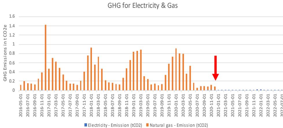
Greenhouse gas (GHG) emissions for natural gas and electricity for ID #019. The red arrow indicates when the heat pump was installed.
