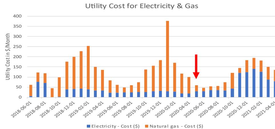
Utility costs for natural gas and electricity for ID #007. The red arrow indicates when the heat pump was installed. A spike occurred in BC Hydro billing at the time of heat pump installation, likely due to fees for BC Hydro equipment upgrades required to support a heat pump. This cost was removed from the data to limit the analysis to operating costs.
