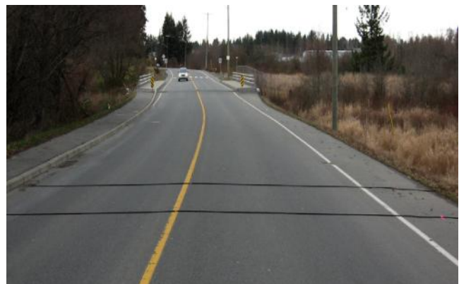
A typical traffic counter installation on Westwood Rd.
