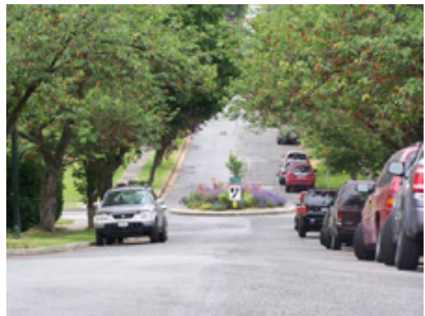
Example of neighbourhood bikeway route with traffic circle to calm vehicle traffic.
