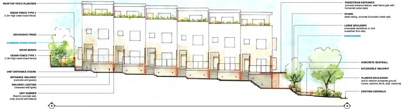
Elevation A South Elevation - Entrance Walkway Scale 1:100
